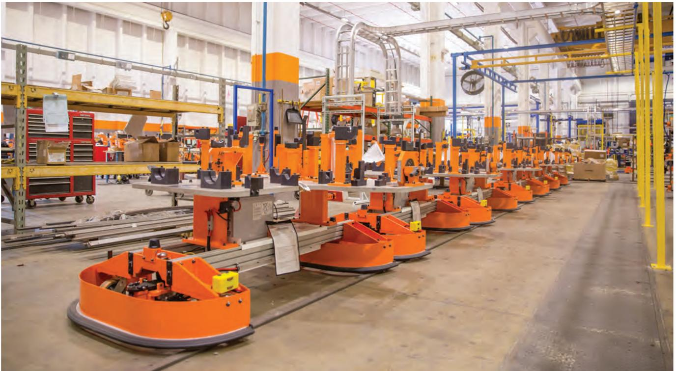
Fori Automation Inc., a specialist in automatic conveying and handling systems, relied on this flexibility while modernizing the assembly line of a large U.S. automobile plant with rail guided carts (RGCs). Each individual RGC has a safety bumper, an emergency stop switch, and optional safety scanners.
